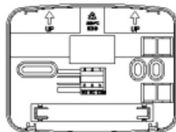
b. Fix the base on wall with provided screws
